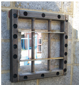
Minimum size grille set up ready for testing of fixing design concept, to determine suitability for reinforced concrete applications.
