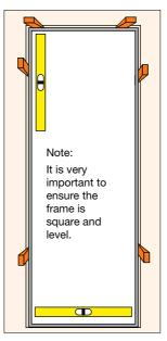
Hold the frame in place using wedges. The wedges must be in line with either the horizontal or vertical members of the frame as incorrect positioning can lead to the frame being bent or distorted.
